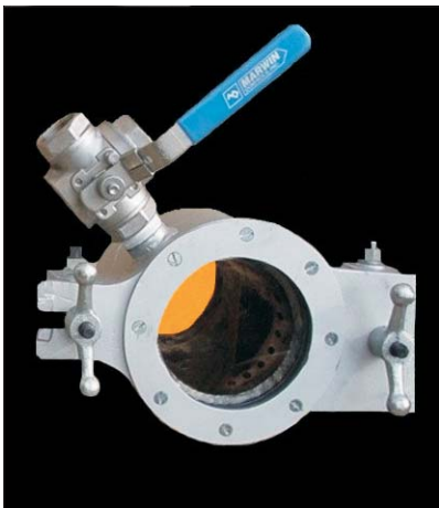
6" Diameter Observation Door for pressurized furnaces complete with aspirating air valve.
