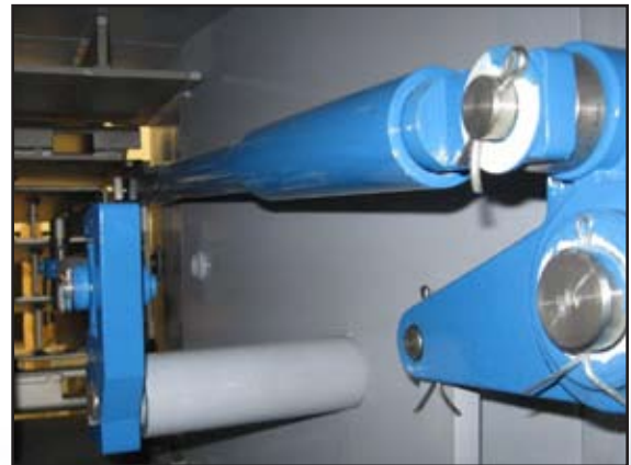
Tilt Mechanism Driving Nozzle Tip Movement
