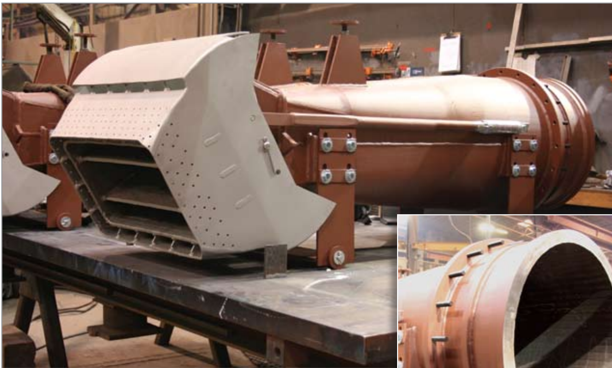
CHROMIUM CARBIDE NOZZLE WITH THERMAL GUARD® II TIP (ABOVE) VIEW OF CHROMIUM CARBIDE LINING (RIGHT)
