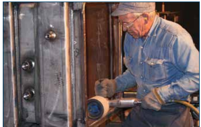
Polishing a Sterilizer Chamber Vessel
