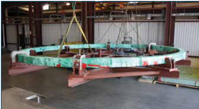
Overhead Cranes Lifting 20' Fabricated Ring
